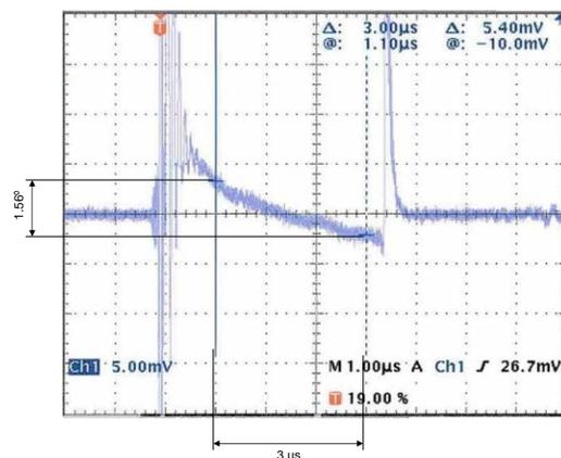
Figure 2: RF phase stability over the  $4 \mu\text{s}$  pulse.
