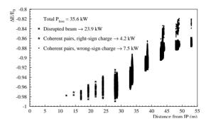
Figure 3: Relative energy spread of the lost particles as a function of the position of loss in the post-collision chicane.
