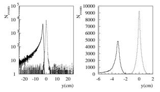
Figure 2: Vertical beam distribution 100 m downstream of the post-collision magnetic chicane, for the disrupted beam (full line), the beamstrahlung photons (dashed line) and the  $e^+e^-$  coherent pairs (dotted and dot-dashed lines).
