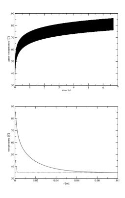
Figure 4: Temperature evolution at the center of the dump window (top) and radial temperature distribution at t = 0 s and t = 6.7 s (bottom).
