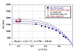
Figure 8: The experimental RF critical field with new shapes.
