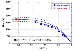
Figure 1: Fitting results of the experimental RF critical field.
