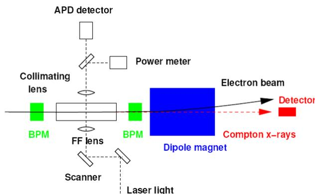
Figure 1: Schematic of the LW IP region.
