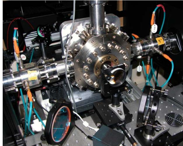
Figure 2: Photograph of the LW vacuum chamber in-situ. Note the two strip-line BPMs, the insertion device for the knife edge (top) and the re-collimation optics.
