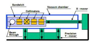
Figure 4: Wakefield Box containing 4 sets of Collimators.
