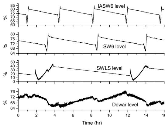
Figure 3: Helium level of magnet cryostats.
