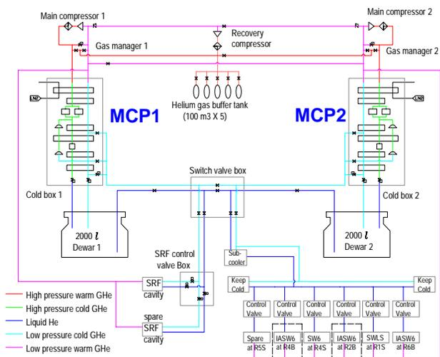
Figure 1: Configuration of cryogenic system.
