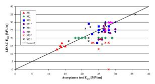
Figure 1: Comparison of the accelerating gradient in the low power acceptance test with the gradient achieved in the machine for each individual cavity.
