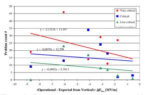
Figure 4: Correlation of the problem count with the difference of the operational gradient of the modules and the average gradient achieved in the acceptance test.
