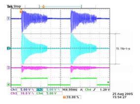
Figure 2: RF envelopes and 50 Hz gate pulse. From top trace, ch.1 driver stage voltage ( $120\times$ ), ch.2 cavity gap voltage ( $1,666\times$ ), ch.3 cavity input current (20A/V) and ch.4 50 Hz gate pulse. 15.1V peak-to-peak at ch.2 corresponds to 12.6 kV peak per gap.
