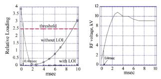
Figure 4: (left) relative beam loading of a second harmonic cavity with and without LOI. (right) required second harmonic voltage per cavity gap.
