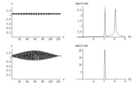
Figure 5: 2D Envelope Oscillations, top  $(x,\varphi)$ , bottom  $(y,\varphi)$ , 20 turns with frequency spectra.
