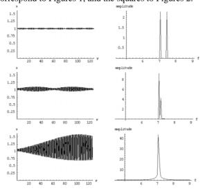
Figure 2: 1D Envelope Oscillations  $(x,\varphi)$ , 20 turns with frequency spectra, approaching resonance. Corresponding parameters are shown in red on Figure 3,  $\Delta Q_e$ =0.01.
