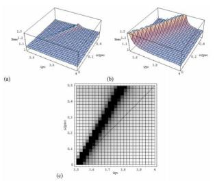
Figure 6: Max. Envelope Amplitudes as a Function of Vertical Set  $(Q_{y0})$  and Depressed  $(\Delta Q_{ysc})$  Tune, for driven  $2Q_y=7$ . (a) is Horizontal  $(x_{max})$ , (b) & (c) Vertical  $(y_{max})$ .
