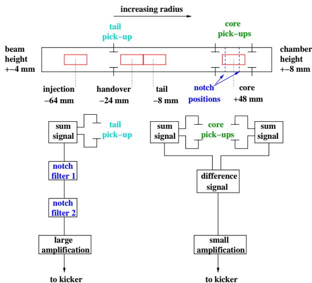
Figure 4: Sketch of pick-up chamber and signal processing. The dispersion at the pick-up is 8 m.
