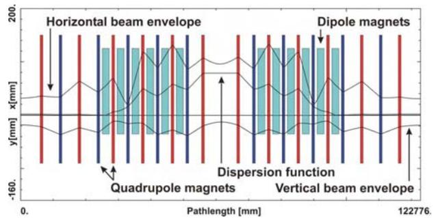
Figure 3: Beam envelopes in the RESR calculated with the MIRKO code.
