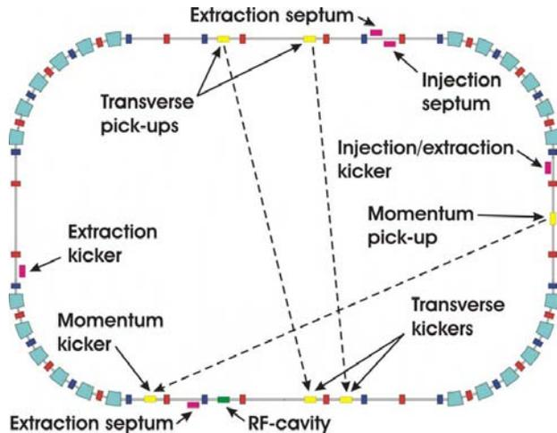
Figure 2: Sketch of the RESR lattice layout.
