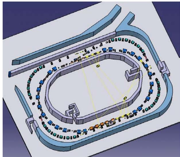
Figure 1: Location of the RESR surrounding the CR storage ring in a common hall. The RESR beam axis is 1.2 m above the CR beam axis.
