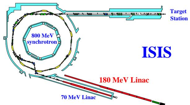
Figure 2: Site layout for the 180 MeV linac.
