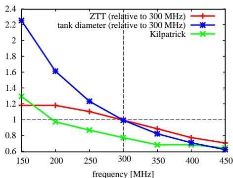
Figure 3: ZTT, Kilpatrick, and tank diameter versus frequency for a DTL cell at: 15 MeV,  $\text{gap}/\beta\lambda = 0.3$ , drift tube face angle: 10 deg, drift tube diameter: 160 mm,  $E_0 = 2.5$  MV/m.
