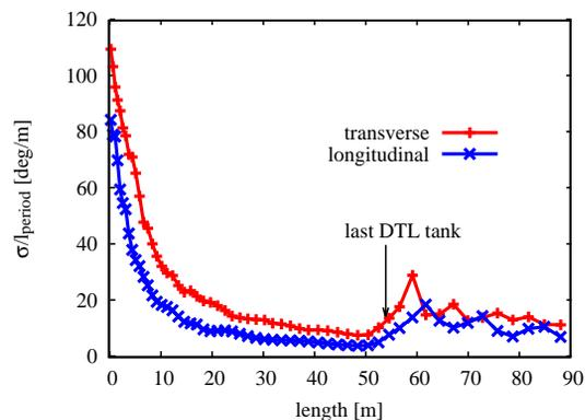
Figure 4: Transverse/longitudinal phase advance per meter.
