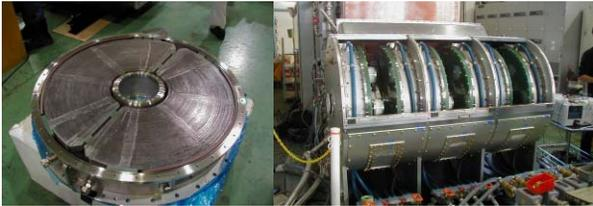
Figure 5: MA cut core (left) and the MA loaded cavity (right).
