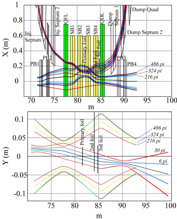
Figure 2: Schematic view of the injection straight in the horizontal (upper) and vertical (lower) plane.
