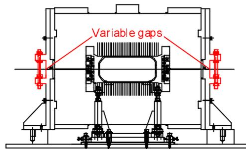
Figure 7: Sub-bending magnet with variable gaps
