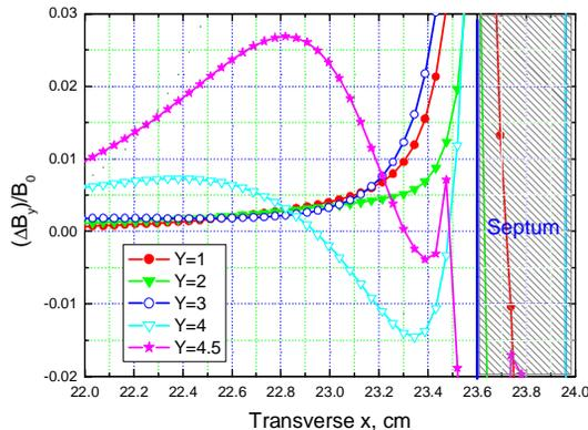
Figure 6: Magnetic field distribution near septum
