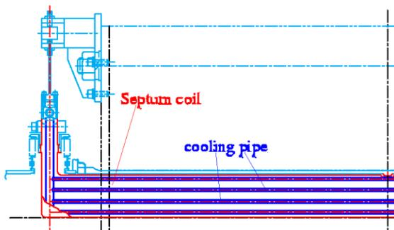
Figure 4: Longitudinal structure of opposite-field septum
