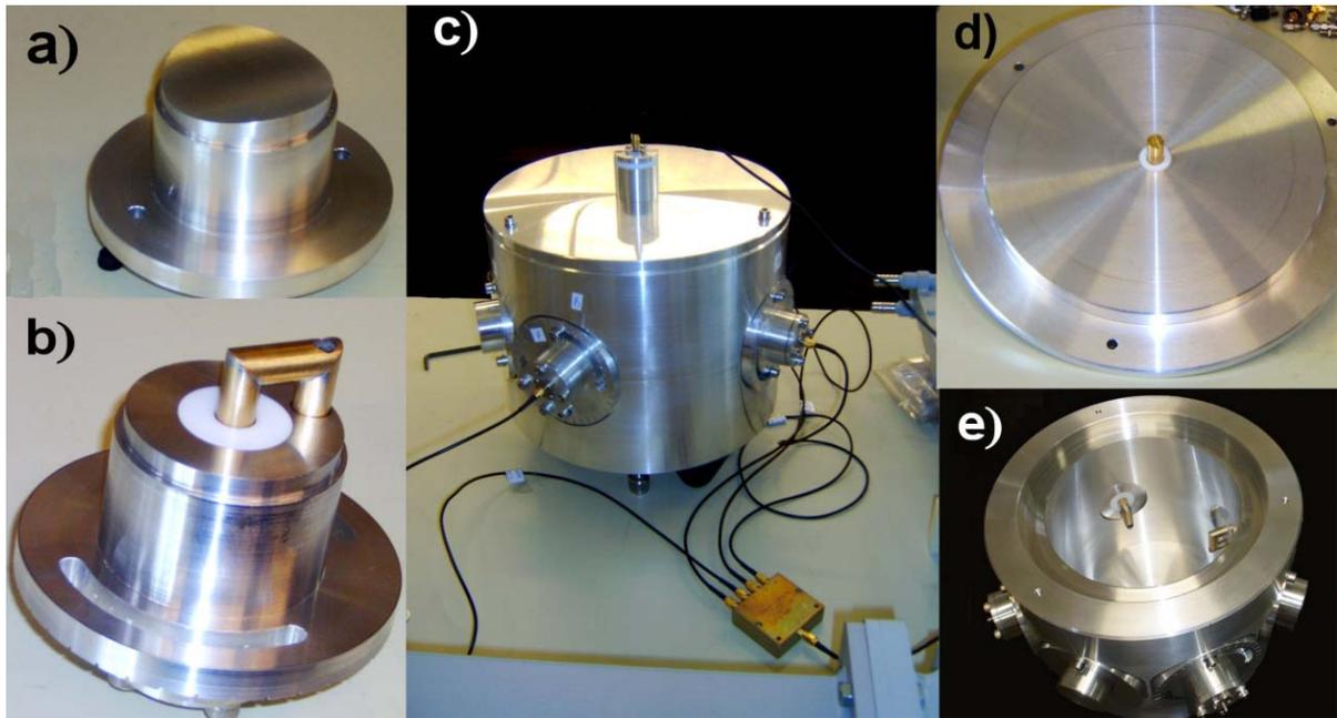
Figure 3: Cavity images a) dummy port, b) port with brass coupler, c) finished cavity d) lid with stub coupler e) inside of the cavity.
