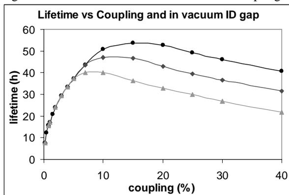
Fig. 4: Touschek Lifetime as a function of coupling for different values of narrow ID half aperture (3.5 mm, black; 3.0 mm red; 2.5 mm green)
