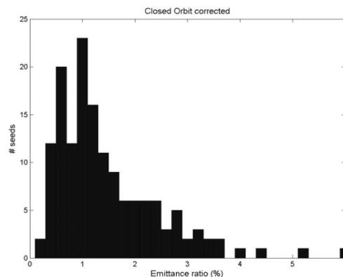
Figure 1: Distribution of emittance ratio  $\chi$  over 150 random seeds, after closed orbit correction.
