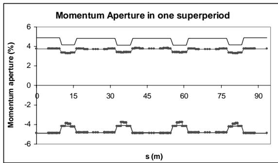
Fig. 3: Momentum aperture in a DIAMOND superperiod with the second order momentum compaction (red line) and without (black line).
