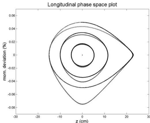
Fig. 2: Longitudinal phase space plots for DIAMOND, with the second order momentum compaction (red line) and without (black line).
