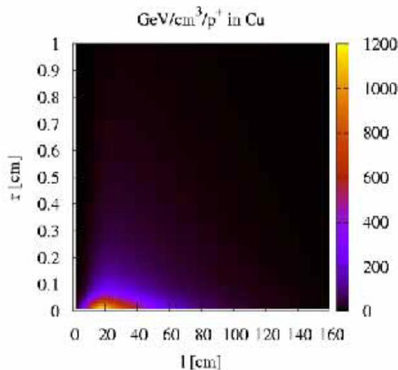
Figure 1: Energy deposition per proton in copper as a function of depth into the target and the radial coordinate.
