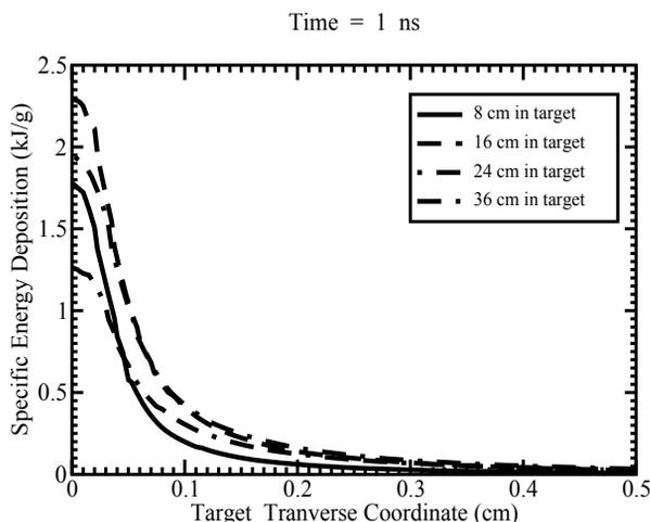
Figure 4: Energy deposition along the transverse coordinate by one bunch at different longitudinal positions.
