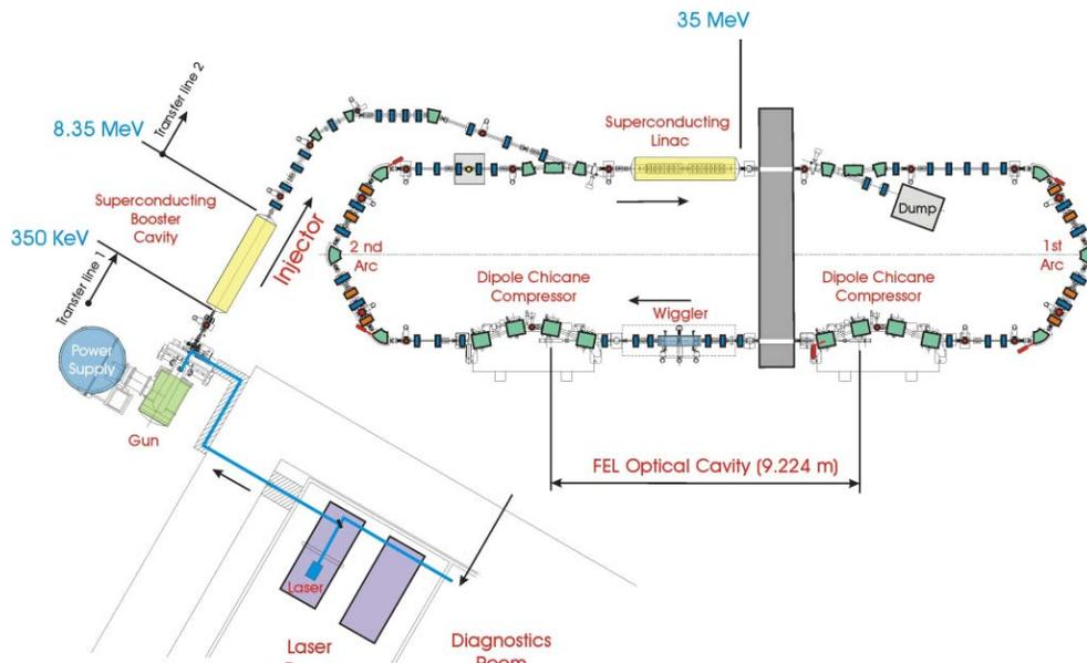
Figure 1: Layout of Daresbury Energy Recover Linac Prototype.
