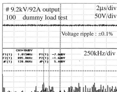
Figure 2: Voltage ripple and its Fourier spectrum
