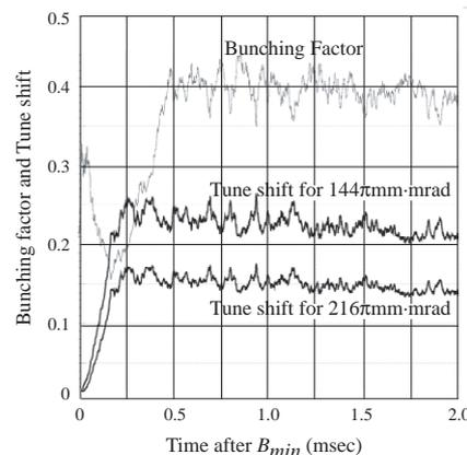
Figure 1: Time variations of the Bunching factor and Tune Shift after the RCS Injection;  $0.25\text{ms}/\text{div}$
