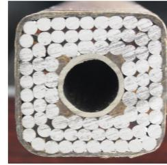
Figure 3: Cross section of an aluminium stranded conductor.
