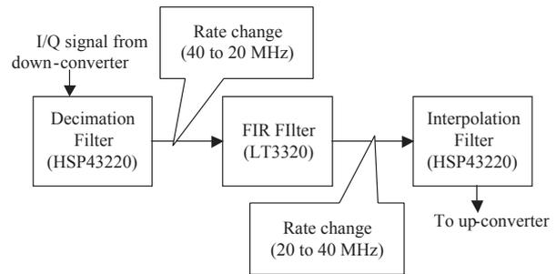
Figure 4: Possible configuration with commercial chips
