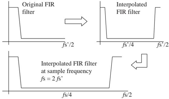
Figure 5: IFIR filter frequency response
