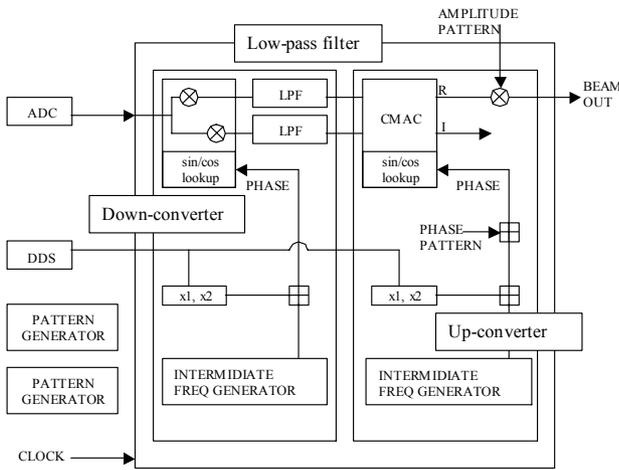
Figure 2: Block diagram of the digital feedforward systems
