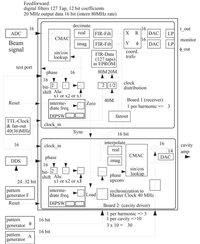
Figure 6: Block diagram of the test module
