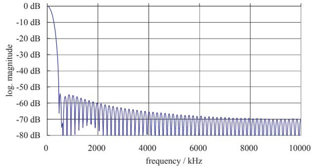
Figure 3: 127-tap FIR filter frequency response, 20MHz sampling rate
