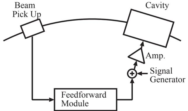
Figure 1: RF feedforward systems
