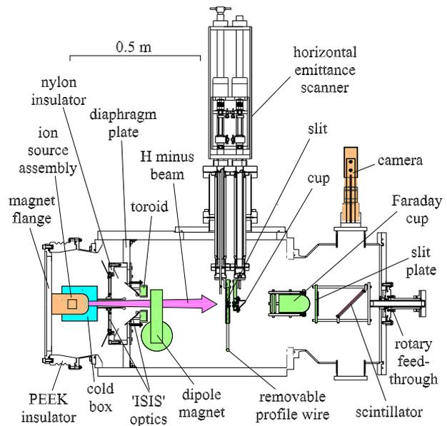
Figure 1. Schematic plan view of the ISDR diagnostics layout, configured for ‘ISIS’ optics.
