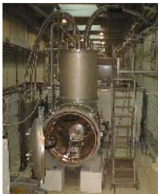
Figure 4: A105 cavity in the CryHoLab test stand.
