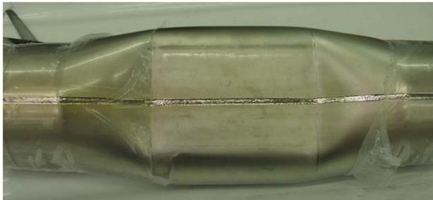
Figure 5 : Spoke bar after forming
