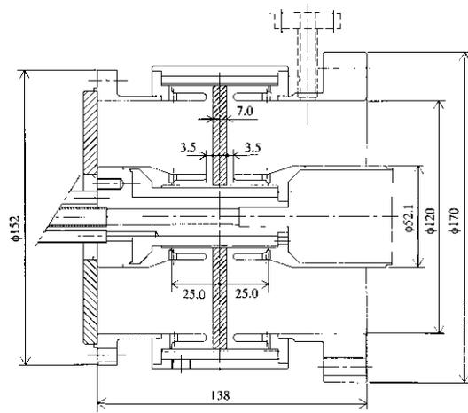
Figure 8: A 972MHz coaxial ceramic window
