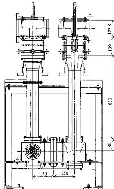
Figure 9: High power test stand for 972MHz input couplers
