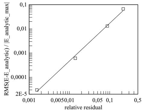
Figure 3: Error of the electric field as a function of the residual.
