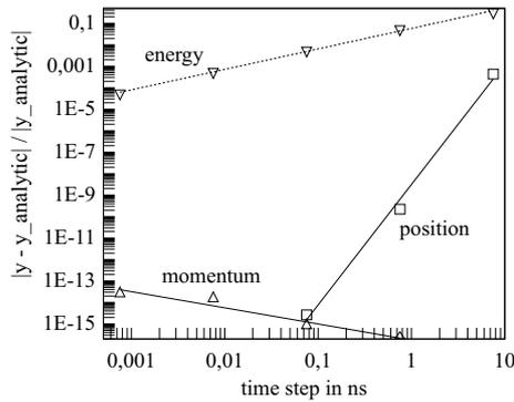
Figure 1: Relative error in space, momentum and energy of a single particle after acceleration within a homogeneous electric field of  $E_z = 250 \frac{\text{kV}}{\text{m}}$  over a distance of 1 m.
