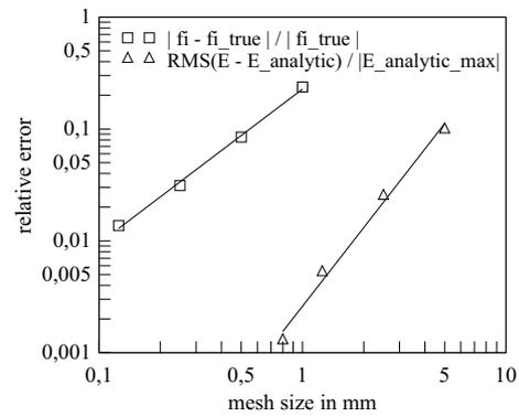
Figure 2: Local discretization error of the potential and the electric field as a function of the mesh size.
