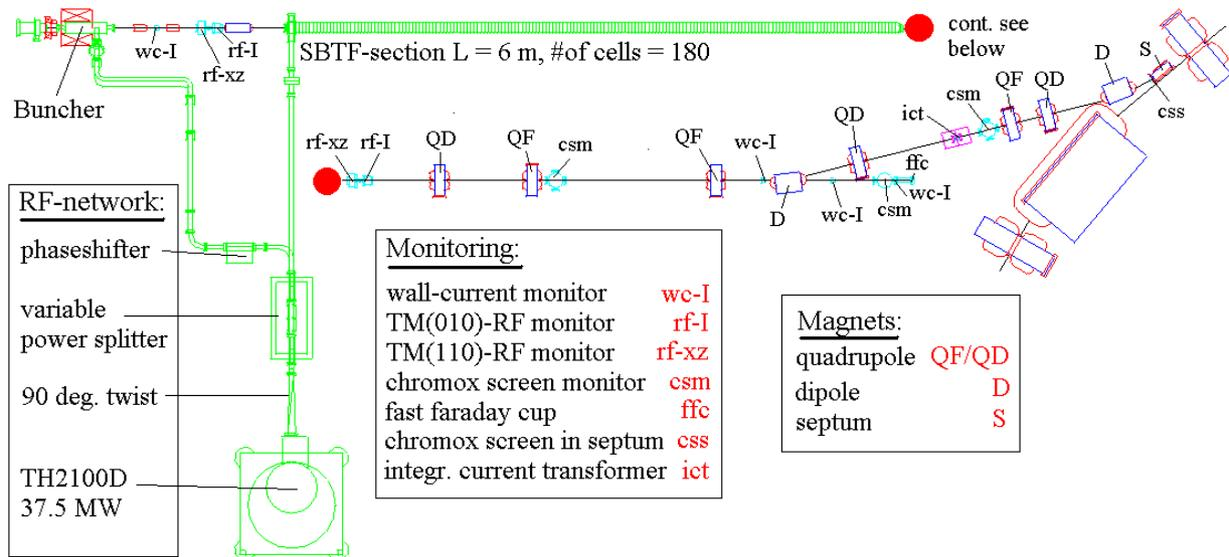
Figure 1: Schematic layout of the new linac system
