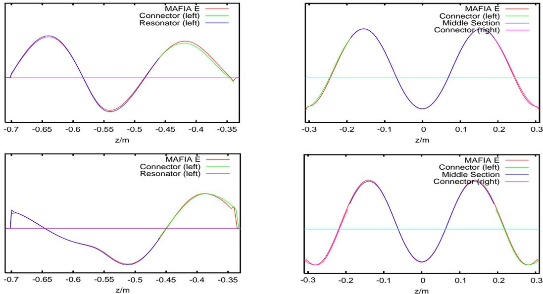
Figure 4:  $E_y$ -component of the eigenmodes with  $f = 1.44258$  GHz (first row) and ( $f = 1.50325$  GHz) (second row) along two path segments perpendicular to the port plane comparing CSC and MAFIA-E.
