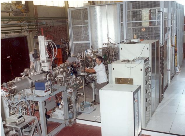
Figure 2 : The high-intensity ECR source SILHI, LEBT and emittance measurement unit
