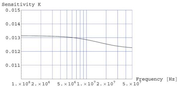
Figure 4: Calculated position response in the frequency domain.
