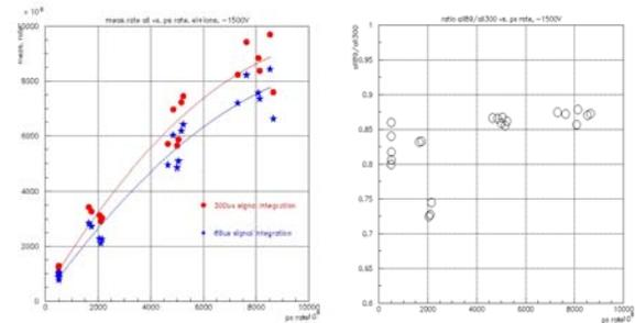
Figure 8: Left: Measured proton intensity vs. PS Booster intensity. Right: Ratio of measured intensity for  $89\mu\text{s}$  and  $300\mu\text{s}$  integration times vs. PS Booster intensity.
