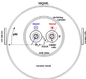
Figure 4: Cross-section of the MQML quadrupole in Q10.
