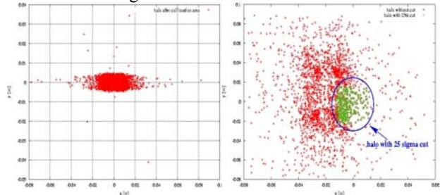
Figure 1: Left: Tertiary halo distribution after the collimation section IR7. Right: Halo tracked with MAD-X to the dispersion suppressor in IR1. Particles with amplitudes larger than  $25\sigma$  are cut.
