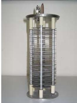
Figure 6: Photo of an ionisation chamber.
