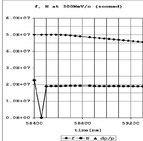
Fig. 3b: zoomed view on the data of Fig.3a (bunched beam) which shows the high temporal resolution for bunched beam measurements.
