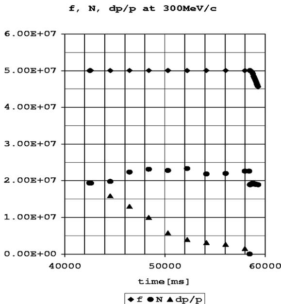
Fig.3a: data taken on 24 Sept 2002 at the end of flat top 300MeV/c: diamonds:  $f_{rev}$  [1/100 Hz]; circles: N [1]; triangles: dp/p [1e-10], injection  $t=0$ . The beam is bunched again at 58460ms.
