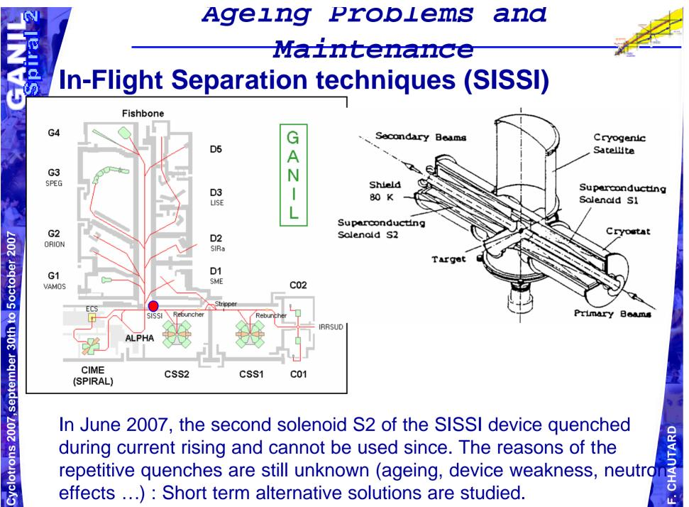
In June 2007, the second solenoid S2 of the SISSI device quenched CHAUTARD during current rising and cannot be used since. The reasons of the repetitive quenches are still unknown (ageing, device weakness, neutro effects ...) : Short term alternative solutions are studied. u.
