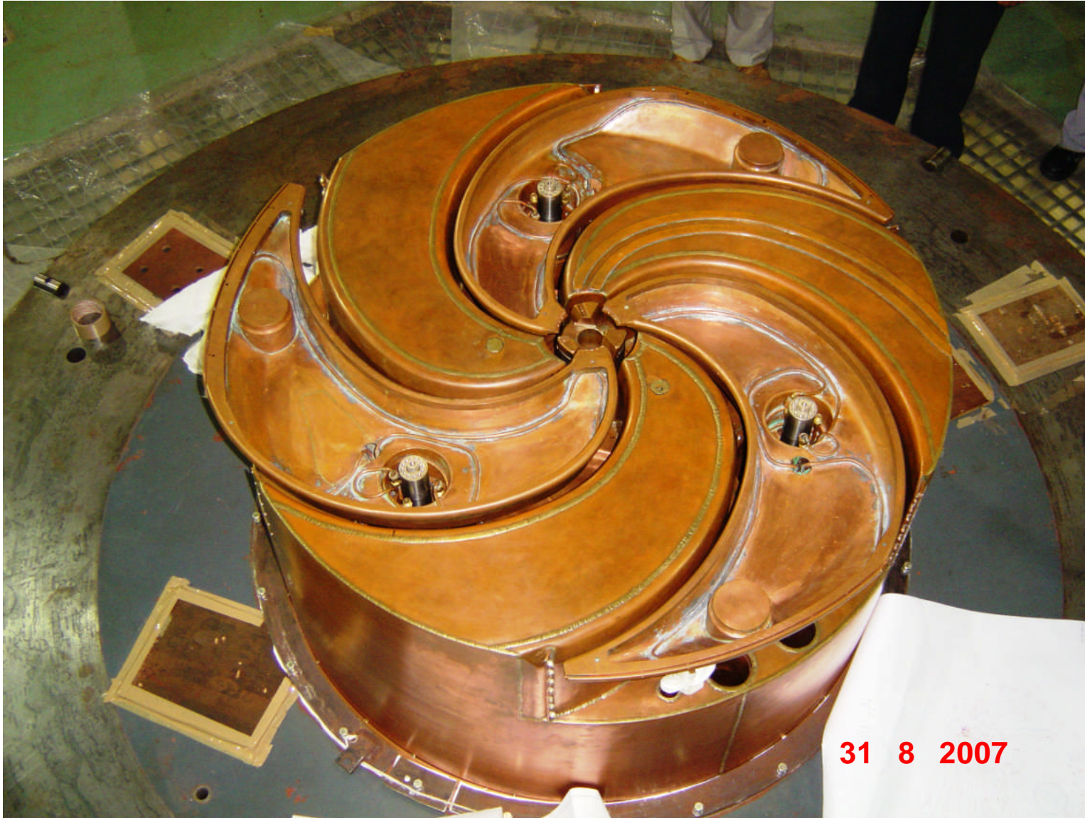
Dees with lower RF liner in position
