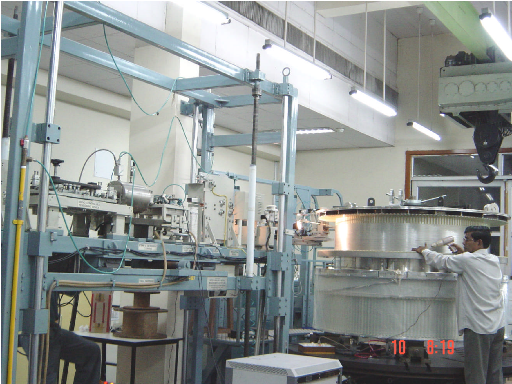
Coil winding in progress
