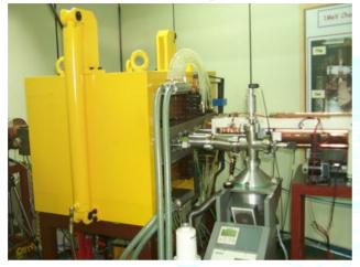
Energy: 1 MeV Particle:proton Beam Current: 100 nA
