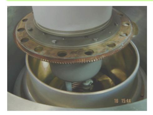
Eimac 4CW 150,000E Tetrode assembled with Blocking Capacitor
