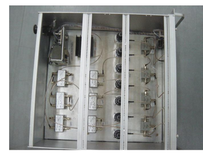
Phase shifting of 120° is done by double mixing and auxiliary transmission line based technique, thereby making insensitive to frequency change
