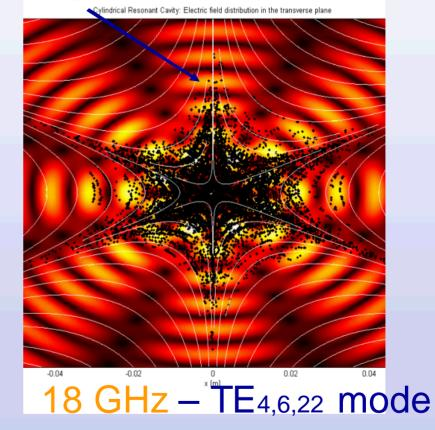
For TE4,4,23 the electric field is five times higher than TE4,6,22 at the resonance
