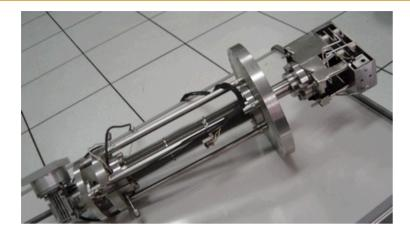
**IMP** Allison-type emittance scanner. Located after the analyzing magnet
