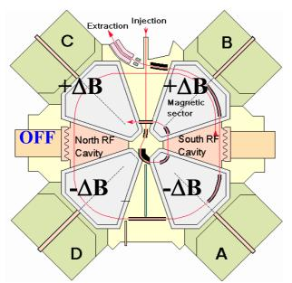
Figure 7: Magnetic field modifications on the SSC ( $\pm\Delta B$ ) to allow the beam extraction with one RF cavity acceleration
