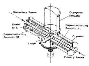
Figure 8: Schematic view of the cryostat of SISSI.
