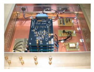
Figure 2: the DDS generator
