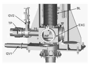
Figure 2: The exchange chamber (EXC) with the front window and lateral door opened, ready for exchange of the spiral inflector (INF); GV1 and GV2 – gate valves, TP – turbomolecular pump, and BL – bellows.
