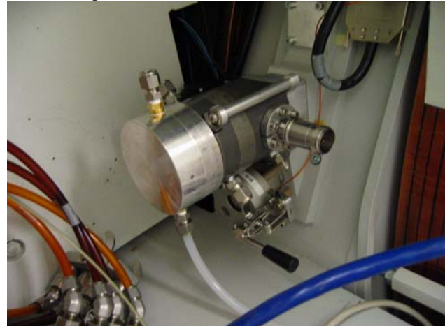
Figure 2: The installed “Short Port” beamline with diagnostic target attached.
