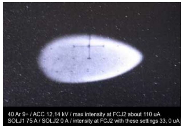
Figure 4: The beam envelope at the beam viewer located after DJ1 (see Fig. 1).
