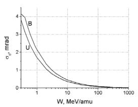
Figure 7. Dependence of the scattering angles for B and U in the carbon foils having the equilibrium thickness
