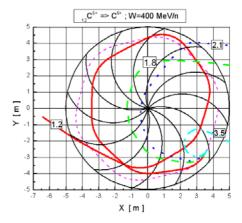
Figure 12. Extraction trajectories by stripping (N6,  $\gamma$ =1.43,  $\xi$ =+45°, flatter=1)
