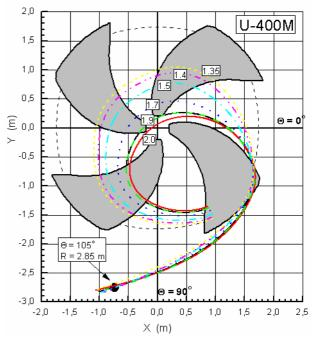
Figure 2. Reference particle trajectories of the ions extracted from U400M cyclotron by method 2
