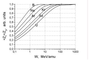
Figure 5. Dependence of the ion stripping degree on the ion energy
