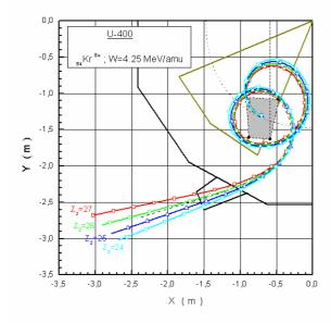
Figure 1. Two-turn extraction from U400 cyclotron
