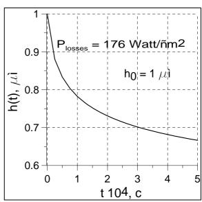
Figure 10. Evolutions of the carbon foil thickness
