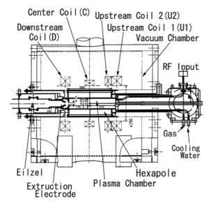
Figure 3: Cross sectional view of liquid-helium free 18 GHz superconducting ECR ion source.
