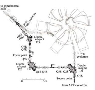
Figure 7: Schematic layout of the beam line to analyze the quality of the beam from the AVF cyclotron as well as to directly deliver low energy and high intensity beams to experimental halls of the ring cyclotron.
