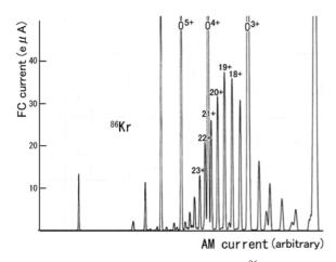
Figure 5: Charge state distribution of <sup>86</sup>Kr ions with 700W RF and oxygen mixing.
