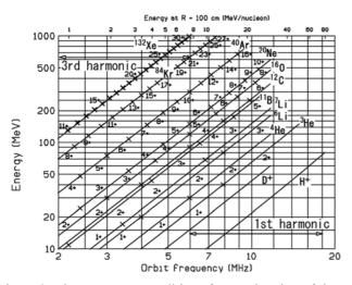
Figure 2: The resonance conditions for acceleration of the RCNP AVF cyclotron.
