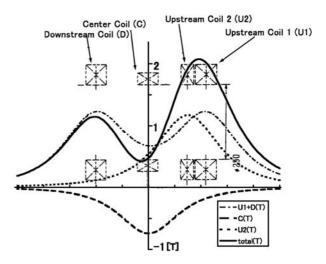
Figure 4: Simulated magnetic field distribution.
