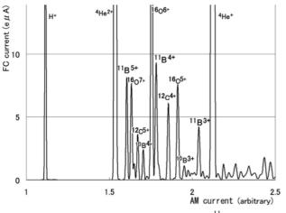
Figure 6: Charge state distribution of <sup>11</sup>B ion.
