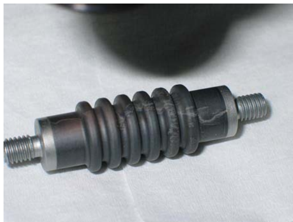
Figure 6: Aluminum nitride insulator with marks from flashover tracks, which are electrically conducting. The insulator body diameter is approximately 1 cm.
