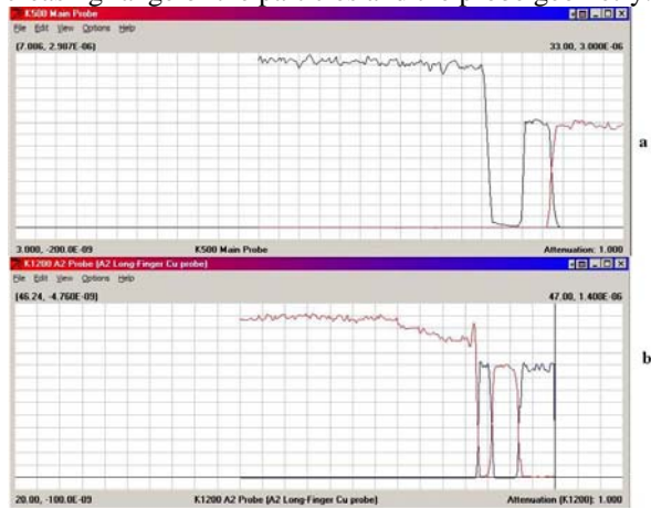
Figure 2: Argon beam probe traces (a) K500 probe, (b) K1200 probe
