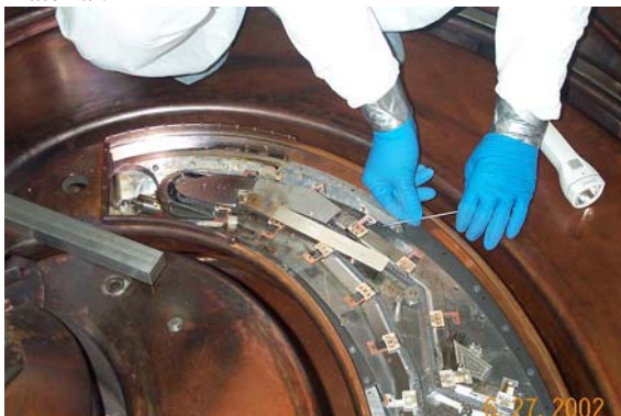
Figure 7: Photograph of the stripper foil mechanism installed in the K1200 cyclotron. Several foils are visible, attached to the chain that transports them into position for use.
