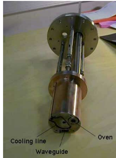
Figure 2: The miniature oven inside the iron plug of the JYFL 14 GHz ECRIS.
