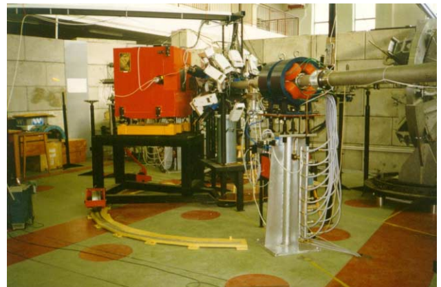
Figure 8. "JANOSIK" a multidetector system dedicated to the investigation of Giant Dipole Resonance
