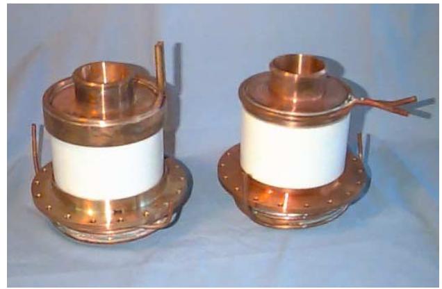
Figure 8: The AAC feedthrough window with and without copper shields covering the metal to ceramic joints.
