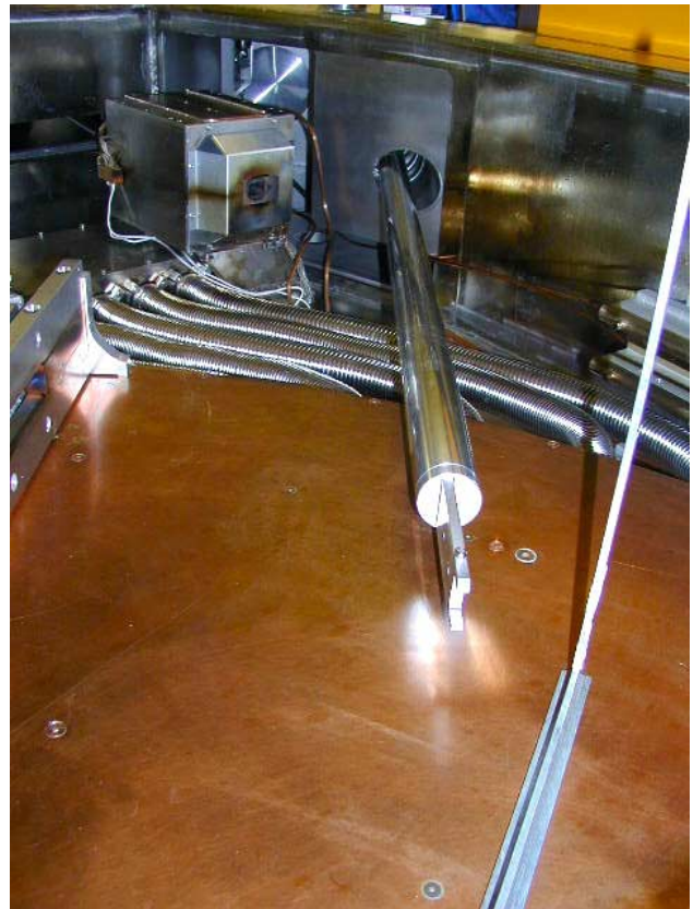
Figure 6. The stripper arm inside the vacuum chamber. The stripper wheel is not in its place.
