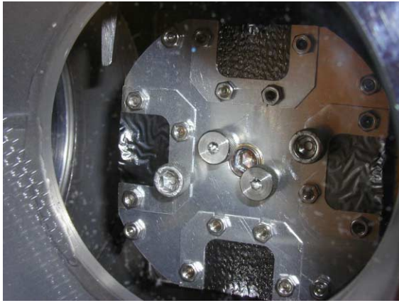
Figure 7. The stripper wheel with four foils as seen through the window in the vacuum lock box. The size of the foil is 16 mm x 22 mm.
