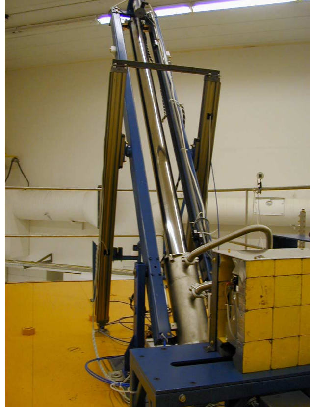
Figure 9. Automatic inflector change system on top of the cyclotron.
