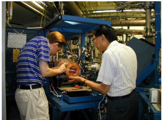
Figure 2. Sami Hahto (JYFL) and Thomas Kuo (TRIUMF) assembling the multicusp ion source.
