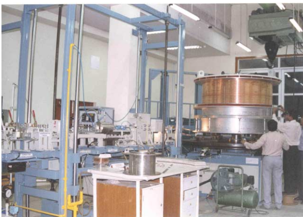
Figure 4 : Superconducting coil winding setup at VECC.
