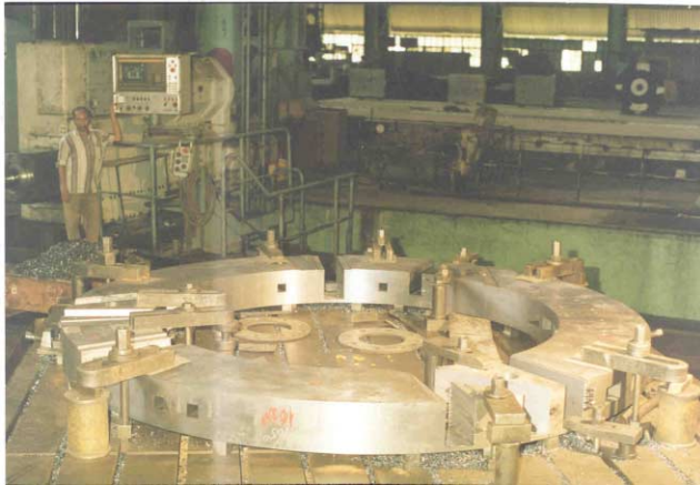
Figure 3 : Machining of the central return path ring for the main magnet frame
